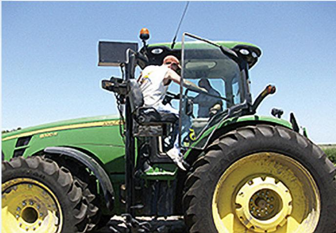
Advanced Mobility Solutions' Ag **Equipment Access Lifts**, available in either platform or seat style, provides access to tractors, combines, or other large equipment.
