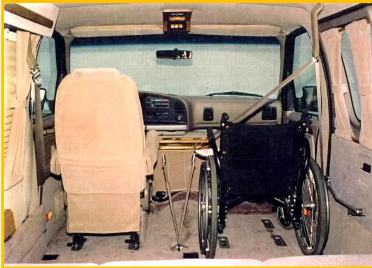
Driver and Front Passenger Lowered Floor
